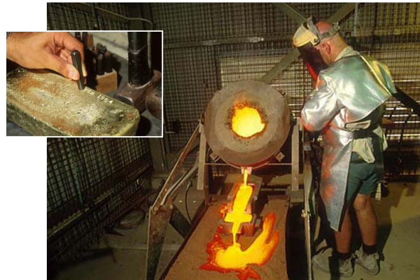
A worker pours liquid Australian gold into a mold to create a standard weight gold bar.
